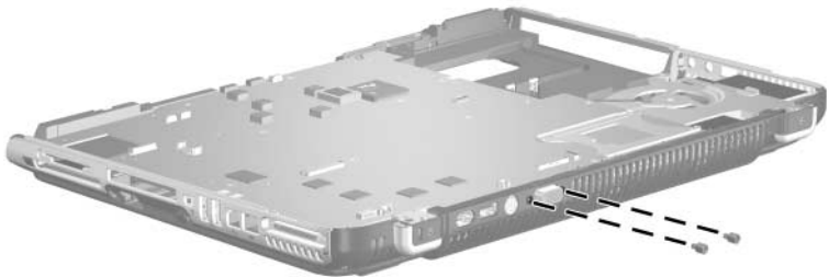
Hex Socket HM5.0×9.0 Screw Lock Locations
