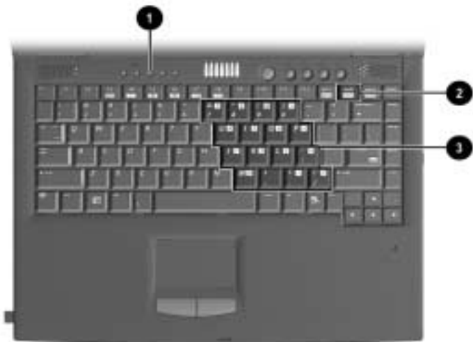
Identifying the embedded numeric keypad
