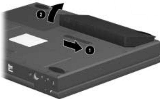
Removing the battery pack
