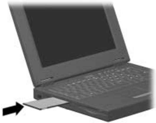
Inserting a PC Card
